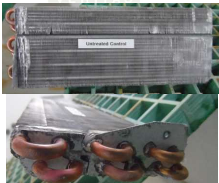
Fig 2: Untreated Control sample after 48 hours neutral salt spray exposure
