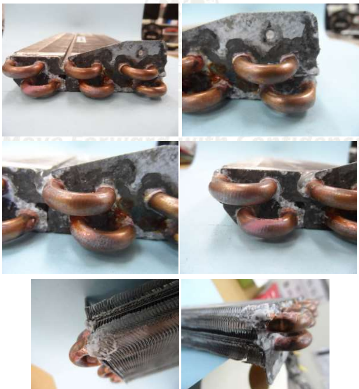
Fig 6: Untreated Control sample after 168 hours neutral salt spray exposure.
