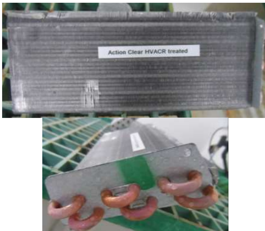
Fig 1: Action Clear HVACR Treated sample after 48 hours neutral salt spray exposure
