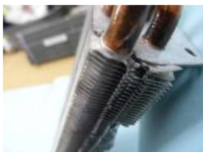
Fig 5: Action Clear HVACR Treated sample after 168 hours neutral salt spray exposure
