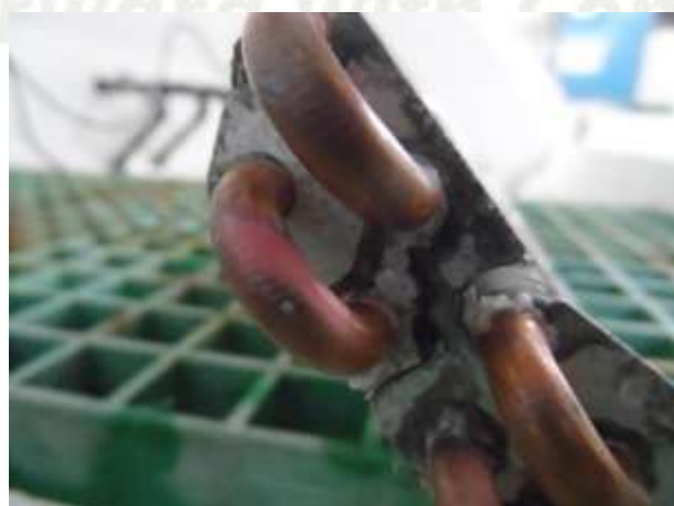
Fig 4: Untreated Control sample after 72 hours neutral salt spray exposure
