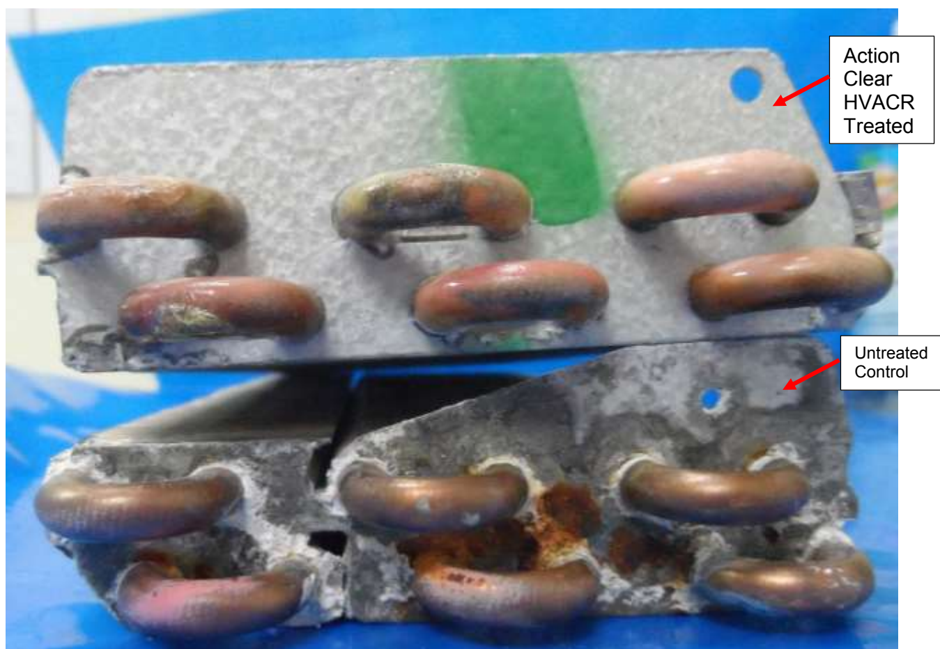
Fig 7: Action Clear HVACR Treated & Untreated Control samples after 168 hours neutral salt spray exposure, Comparison of end plates.
