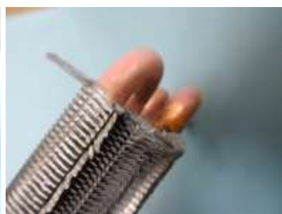
Fig 5: Action Clear HVACR Treated sample after 168 hours neutral salt spray exposure
