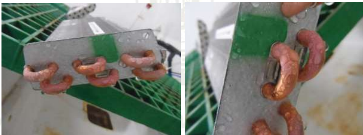
Fig 3: Action Clear HVACR Treated sample after 72 hours neutral salt spray exposure
