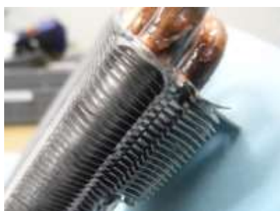
Fig 5: Action Clear HVACR Treated sample after 168 hours neutral salt spray exposure
